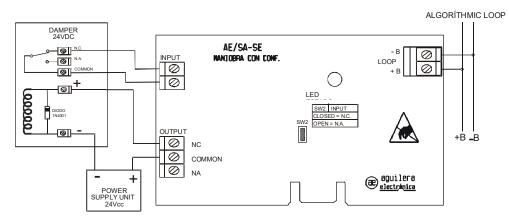
A damper has been shown that needs to be continually fed. If it is desired to connect a damper that needs voltage to close, the positive of the solenoid valve has to be connected to the normally open (NA) contact of the module output.
